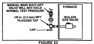
NOTE - Install a 1/8 inch NPT plugged tap in the field piping upstream of the gas supply connection to the unit. The tap must be accessible for test gauge connection. See figure 24.
